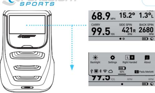
On your GC3 display, swipe down to access the Quick Settings page. On the Quick Settings display, you can access the **BACKLIGHT, SETTINGS, LEFT/RIGHT-HANDED** modes, **ABOUT**, and you can check the battery life
