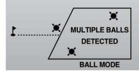
Place the ball on the ground in front of your GC3. If the ball is outside of the hitting zone, you will see the MOVE BALL INTO HITTING ZONE display. If there are multiple balls in the hitting zone, you will see the MULTIPLE BALLS DETECTED display. Once the ball is in the hitting zone, the GC3 will display the READY screen and the LED light will change from blinking to solid
