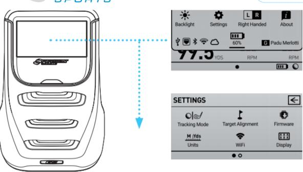
To activate target alignment, swipe down to access the Quick Settings page. Select **SETTINGS**, then go to **TARGET ALIGNMENT**
