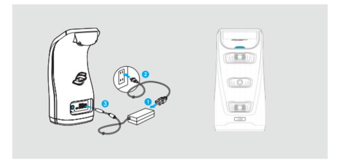
You can use your GC3 right out of the box, but it is recommended that you plug in your GC3 and allow the battery to fully charge before use.
